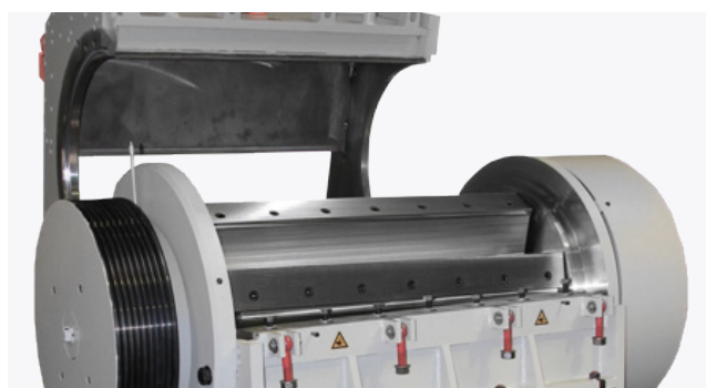
Knife made of high quality, hardened tool steel (Illustration exemplary)
